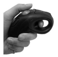
Fig. 2. The hand-held finger mouse used in the experiment
